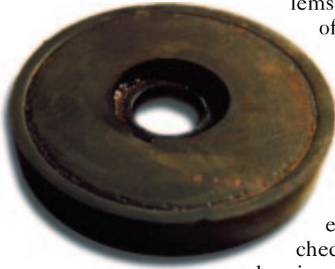
When testers come across problems during the field test of a backflow preventer, they normally try to assess the situation to determine the problem. Often when a tester obtains an inadequate reading on a check valve, the problem is merely debris which was caught on the disc. This is cleaned off, the assembly reassembled and re-tested.
