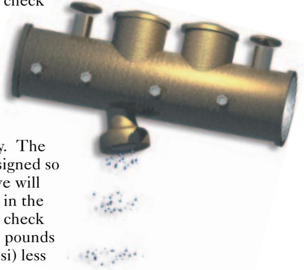
**When the relief valve discharges intermittently, the RP is most likely doing exactly what it is designed to do.**
