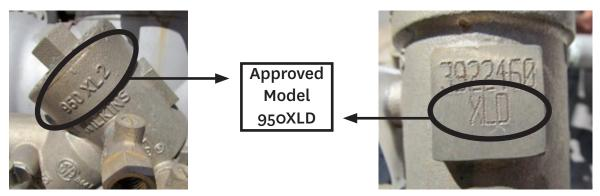
Assemblies marked as illustrated above are considered Approved Model 950XLD assemblies. As of 16 September 2014, and starting with serial number 3981297, the model designation "950XLD" is only cast on both sides of the first check valve body.
