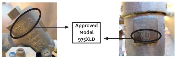
Assemblies marked as illustrated above are considered Approved Model 975XLD assemblies. As of 16 September 2014, and starting with serial number 3981297, the "975XL2" remains cast into the body and the "975XLD" model designation is stamped on the flat boss below the serial number on the body.
