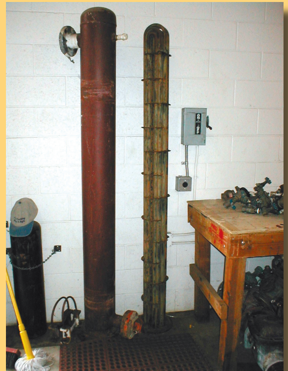
Internals of a Heat Exchanger
